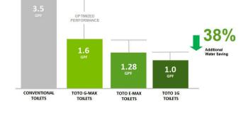
flushing systems, such as Tornado Flush $^{\!\scriptscriptstyle \mathsf{T}\!\mathsf{M}}$  and Siphon Jet Flush, reinforce TOTO's performance reputation while offering an additional water savings of 20% and 38% respectively.
