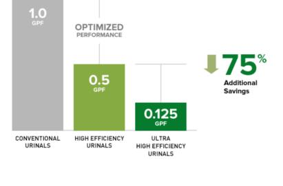
Designed to work in combination with the EcoPower® Ultra High-Efficiency Urinal Flush Valve, the 0.125gpf urinal reinforces TOTO's performance reputation while offering an additional water savings.
