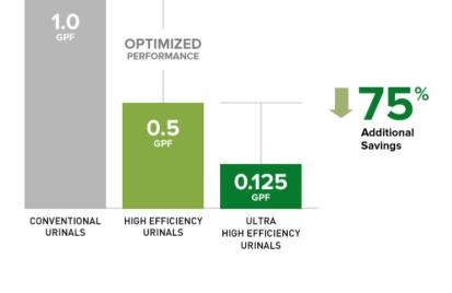
Designed to work in combination with the EcoPower® Ultra High-Efficiency Urinal Flush Valve, the 0.125gpf urinal reinforces TOTO's performance reputation while offering an additional water savings.
