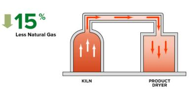
Waste heat from the kilns is routed to the product dryer. This reduces 15% natural gas consumption.
