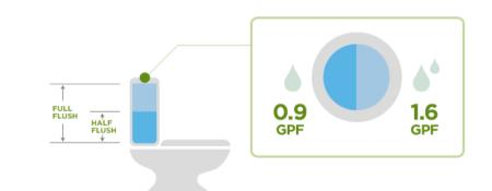
The dual flush system reduces water in the use phase.
