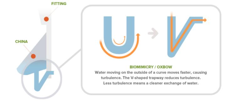
biomimicry, modeled after the oxbow effect found in nature. Water moving on the outside of a curve will move faster, causing turbulence. The 0.125gpf urinal utilizes a V-shaped trap to reduce turbulent flow, resulting in lower water use without compromising performance.
