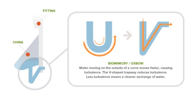
Designed to work in combination with the 0.125gpf urinal, the flush valve is engineered to utilize biomimicry, modeled after the oxbow effect found in nature. Water moving on the outside of a curve will move faster, causing turbulence. The 0.125gpf urinal utilizes a V-shaped trap to reduce turbulent flow, resulting in lower water use without compromising performance.
