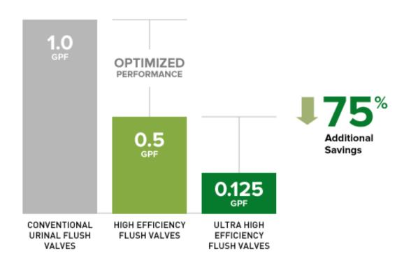
Using our proven EcoPower engineering, the 0.125 gallon per flush urinal flush valve reinforces TOTO's performance reputation while offering an additional water savings.
