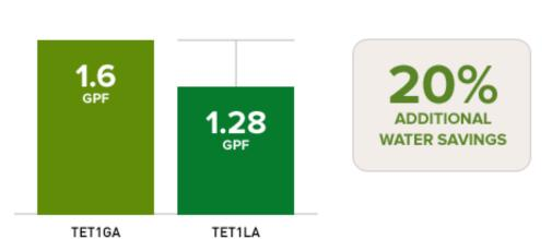
Using the same proven engineering as our legendary EcoPower TET1GA, the TET1LA high-efficiency toilet flush valve reinforces TOTO's performance reputation while offering an additional water savings.
