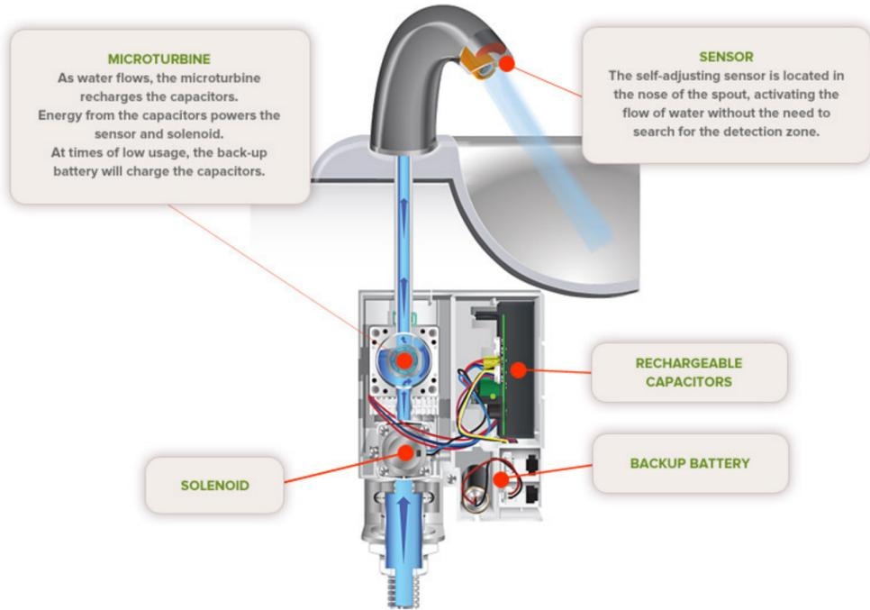
**SENSOR:** Located in the nose of the faucet, the EcoPower sensor ensures that water flows only when needed. The detection zone is right where you need it, eliminating the need to search with your hands to activate the flow of water. For on-demand versions, the sensor will stop the flow of water upon removal of the hands from the sensing zone, preventing wasted water.
