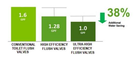
Using the same proven engineering as our legendary EcoPower conventional and high-efficiency toilet flush valves, the ultra-high efficiency flush valve reinforces TOTO's performance reputation while offering an additional water savings of 20% and 38%, respectively.
