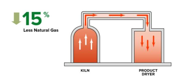
Waste heat from the kilns is routed to the product dryer. This reduces 15% natural gas consumption.
