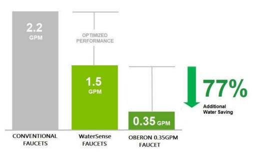
Utilizing the same proven engineering as our high efficiency faucets, 1.5gpm and 1.2gpm, the 0.35gpm Oberon Faucet reinforces TOTO's performance reputation while offering additional water savings of 77% and 71% respectively.
