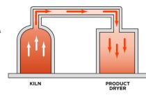
Waste heat from the kilns is routed to the product dryer. This reduces 15% natural gas consumption.
